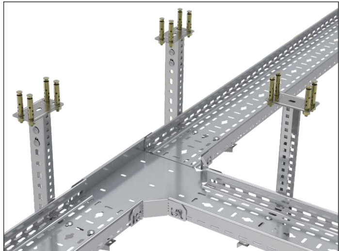
Central support not required on 300mm radius fittings
