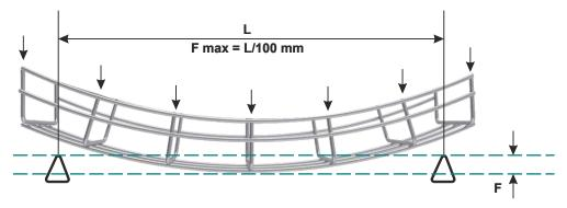
On supports, maximum F deformation and twisting occurs at the ends. The standard requires that the maximum F = L/20 mm. The deformation, F is called deflection, and is expressed in mm.
